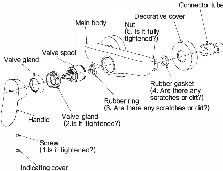
The diagram shows the disassembled parts of a faucet. Labels indicate the Main body, Connector tube, Decorative cover, Nut (5. Is it fully tightened?), Rubber gasket (4. Are there any scratches or dirt?), Rubber ring (3. Are there any scratches or dirt?), Valve spool, Valve gland (2. Is it tightened?), Handle, Screw (1. Is it tightened?), and Indicating cover.
